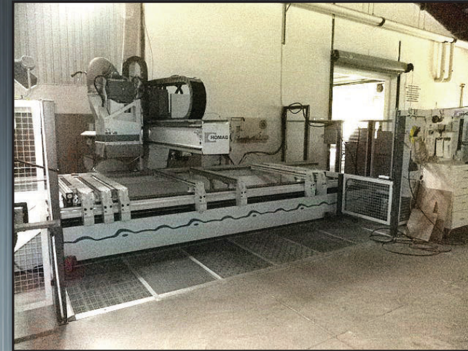
HOMAG OPTIMAT MODEL BAZ322/40/K CNC MACHINING CENTER , S/N 0-201-03-7217 (2004), HOMAG GQ CTRL, ATC, VACUUM LOADING SYSTEM, ASST'D TOOLING
